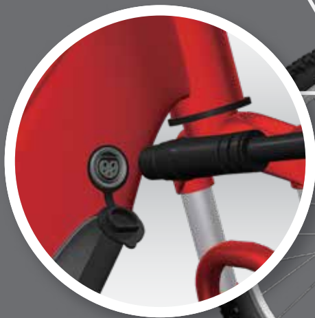
② Battery Charger
