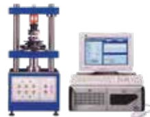
Vertical Tensile Strength Testing
